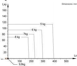
The LBR iisy 8 R930 is designed for a rated payload of 8 kg in order to optimize the dynamic performance of the robot. The maximum payload of 9.6 kg only applies if the position of the center of mass is 0 mm. The specific load case must be verified using KUKA.Load or KUKA Compose. For further consultation, please contact KUKA Support.
