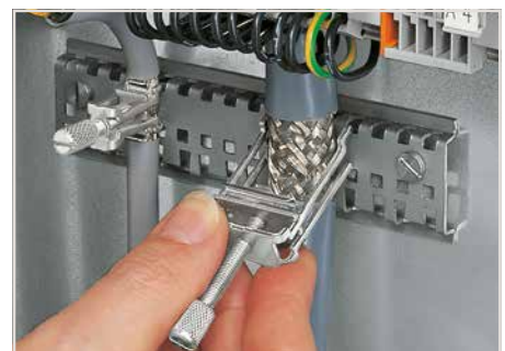
To remove the clamping saddle, unscrew until ratcheted mechanism is released, then slightly tip saddle and remove the clamping saddle.
