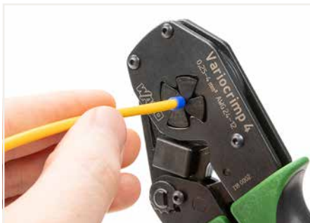
Squeeze handles until ratchet mechanism is released.
