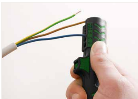
Stripping the conductor insulation
