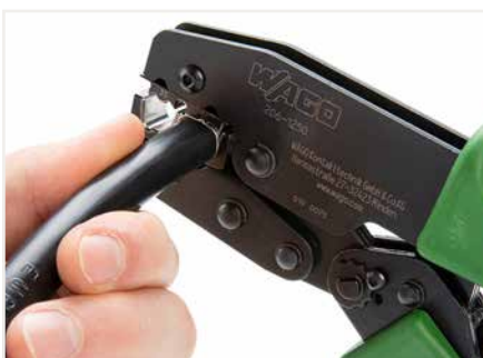
Squeeze handles until ratchet mechanism is released.
