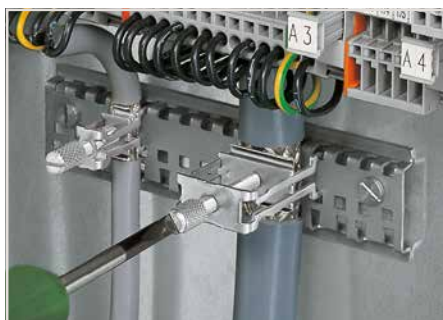
After connection, tighten the knurled screw to complete the installation. Recommended tightening torque: 0.5 Nm
