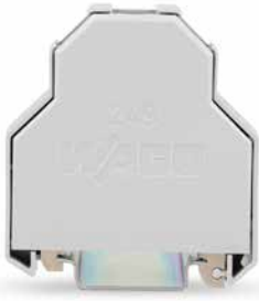
Screwless end stop; 14 mm wide (max. 16.5 mm); for 35 x 15 and 35 x 7.5 DIN-rails
