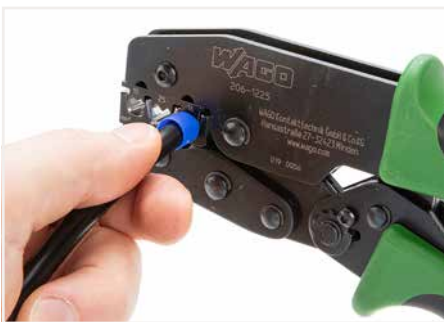
Insert the ferruled conductor into the crimping station.
