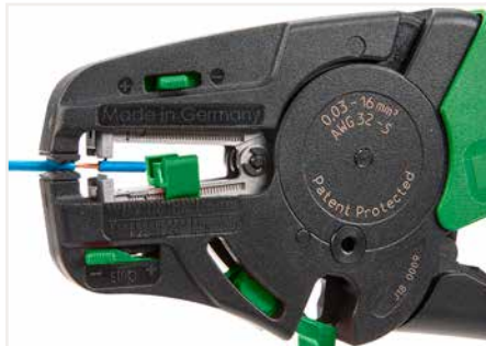
Partially stripping a conductor.
