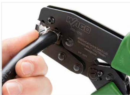
Squeeze handles until ratchet mechanism is released.
