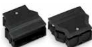
Strain relief housing; Connectable sheathed cable diameter: 9 ... 13 mm; Strip length (outer insulation): 55 mm
