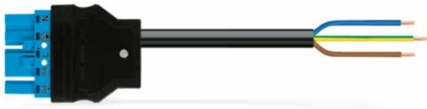
Adapter cable ▶ plug – free end ▶ Sheathed cable diameter: 7.4 ... 9.4 mm ▶ H05Z1Z1-F 3G1.5
