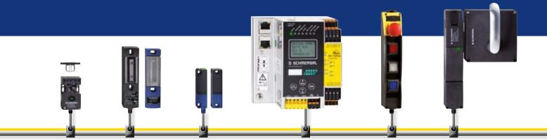
AS-Interface Safety at Work (AS-i Safety) is a safe bus system designed in accordance with the open AS International standard. Safety components such Emergency-Stop buttons, safety switches, solenoid interlocks and safety light curtains are connected via the unshielded 2-wire line of the AS interface which also supplies the components with energy.
