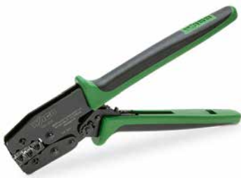
Crimping tool 25; for insulated and uninsulated ferrules; crimping range: 10 mm² (8 AWG), 16 mm² (6 AWG) and 25 mm² (4 AWG)
