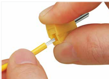
Conductor termination: Press button fully, insert stripped conductor into square entry and release.
