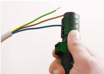
Stripping a conductor insulation.
