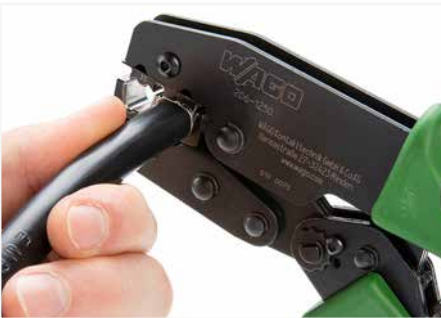
Squeeze handles until ratchet mechanism is released.
