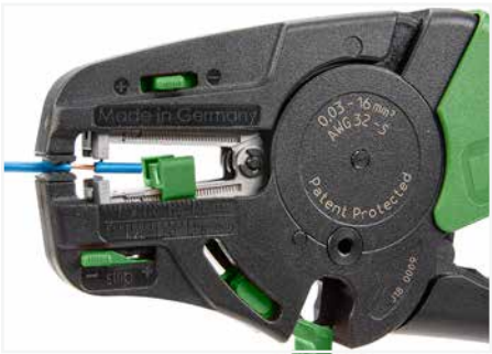
Partially stripping a conductor.
