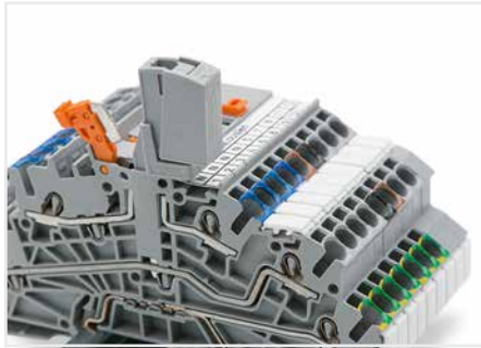
For multilevel installation terminal blocks with internal N-disconnection, test plug adapters can be inserted into the free vertical test slot when the N-potential is disconnected.
