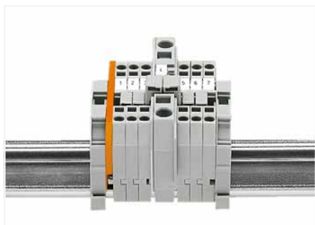
Commoning from 6 mm²/10 AWG (282 Series) to 1.5 mm²/16 AWG (279 Series) rail-mount terminal blocks via step-down jumpers.
