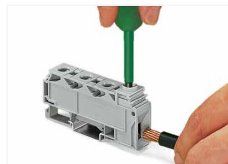
Terminating a 35 mm 2 (2 AWG) conductor – screw clamp connection, side-entry wiring
