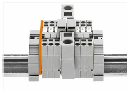
Commoning from 16 mm²/6 AWG (283 Series) to 4 mm²/12 AWG (281 Series) rail-mount terminal blocks via step-down jumpers.
