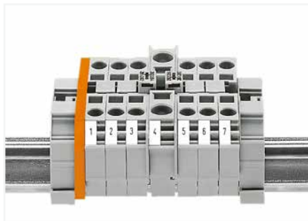
Commoning from 10 mm²/8 AWG (284 Series) to 6 mm²/10 AWG (282 Series) rail-mount terminal blocks via step-down jumpers.
