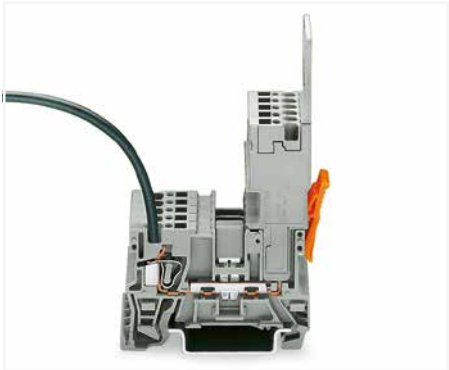
1-conductor/1-pin carrier terminal block (769-176) Conductor cross section: 4 mm² (12 AWG) 1-conductor female plugs (769-102 to 769-115) Conductor cross section: 4 mm² (12 AWG) Conductor loop length: 1 m
