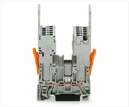
2-pin carrier terminal block (769-156) 1-conductor female plugs (769-102 to 769-115) Conductor cross section: 4 mm² (12 AWG) Conductor loop length: 1 m
