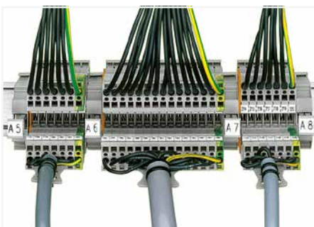
Cable entry into the control cabinet: The cables are led into the control cabinet with the connected female plugs and are directly plugged onto the carrier terminal blocks.
