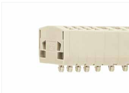
Ex e II terminal strip; with snap-in mounting feet; for 0.6 ... 1.2 mm plate thickness; 3.5 mm mounting hole diameter
