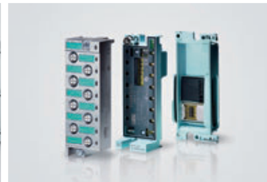
Three-part expansion module: connection, electronics and bus modules
