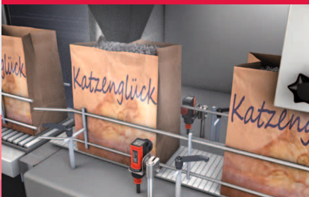
Object detection in bulk material filling
