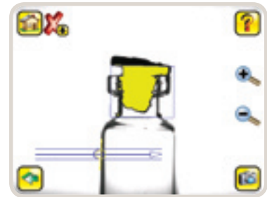
Area with Motion (Vial Stopper Inspection)
