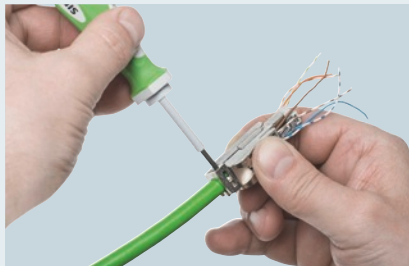
Fasten the casing using a screwdriver
