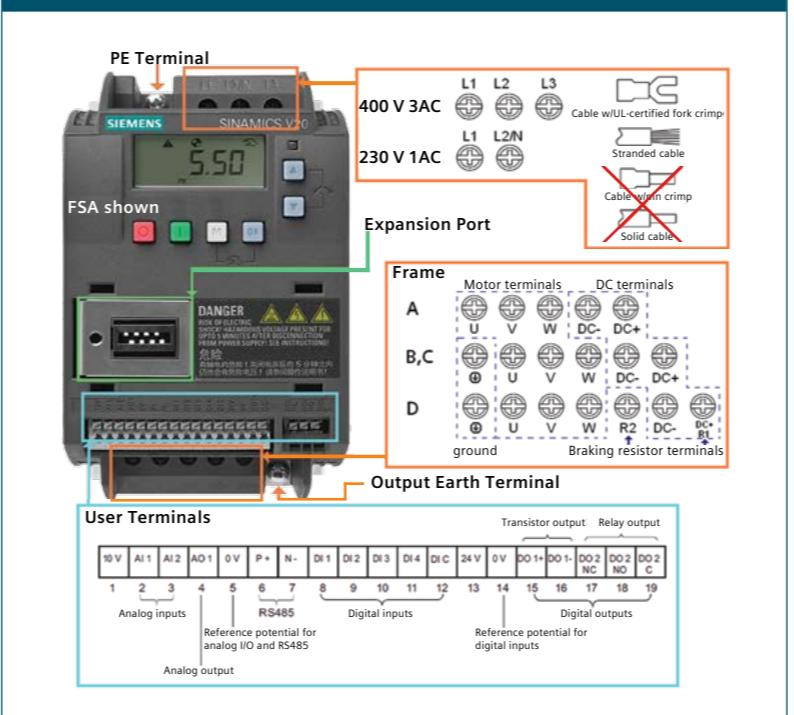
Recommended fuse types for different frame sizes can be found in Section 2.2 (page 6) of the SINAMICS V20 Getting Started Manual.
