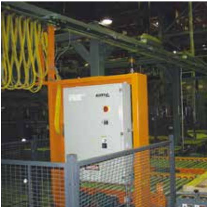
WCS/PCV linear feedback ensures material handling system transfer cars allocate their pallets to the correct conveyor.
