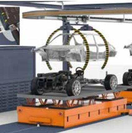
Data matrix control codes initiate decisions at work stations and "Y" branches.
