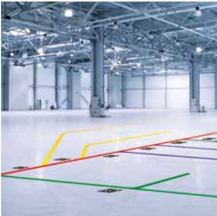
AGV movement is controlled by scanning tapes and painted strips.
