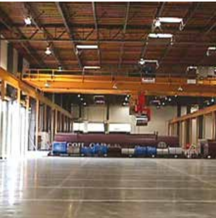
Overhead cranes rely on WCS/PCV for "X" and "Y" positional tracking as well as prevention of skewing.
