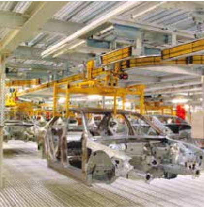
WCS/PCV provides continuous positional feedback of the car body throughout the assembly process.
