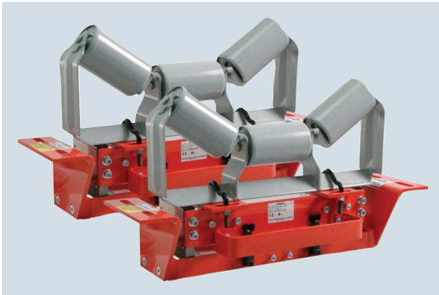
Milltronics MMI is a heavy-duty, high accuracy multiple idler belt scale used for critical process and load-out control. Idler not included with belt scale.
