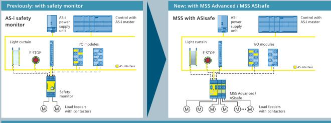
Safety technology with MSS and clever AS-Interface standard
